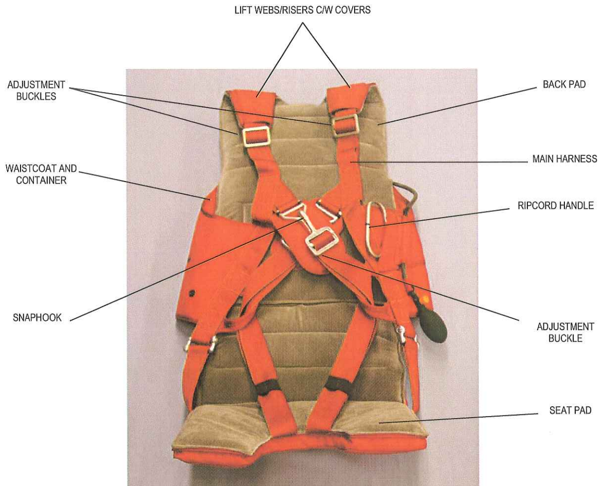
Fig 1 GQ 650 "Silhouette" parachute assembly
