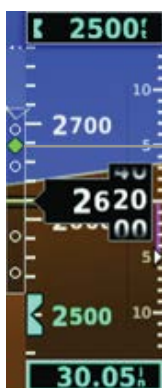
Figure 2-23 Vertical Deviation Indicator (Glideslope ILS Source) - PFD
